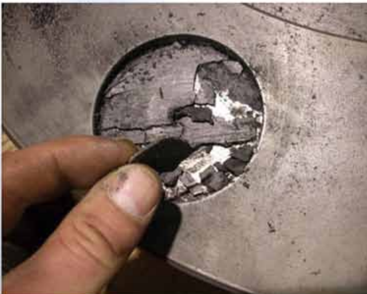
Worn-out viscous damper showing dried silicone flakes. Silicone should be clean and fluid.
