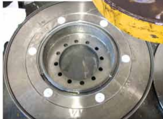
Picture shows a damper with silicone that is still clear and fluid.
